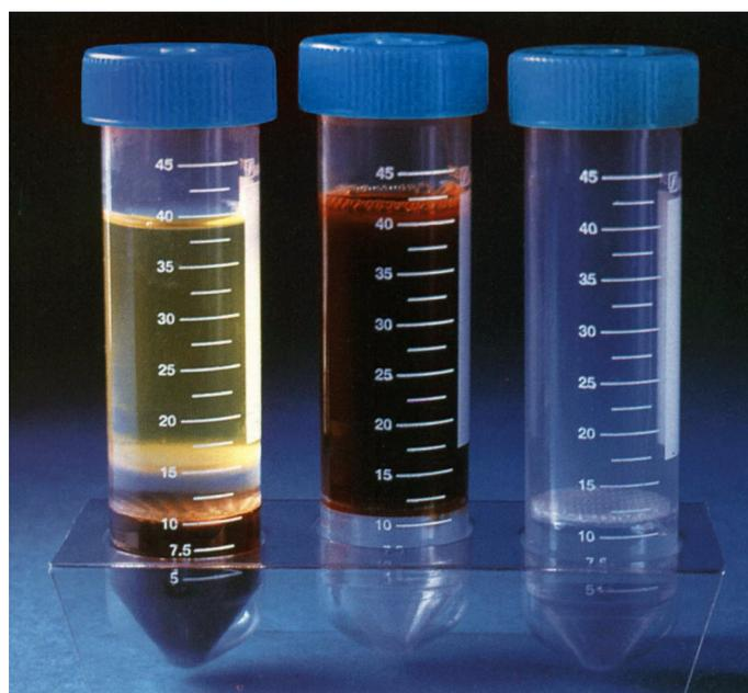
**Lymphoprep™ Tube** is a sterile tube in which the Lymphoprep™ is contained below a plastic filter disc. This allows diluted blood to be poured simply and directly into the tube, the disc preventing any mixing with the separation medium.
