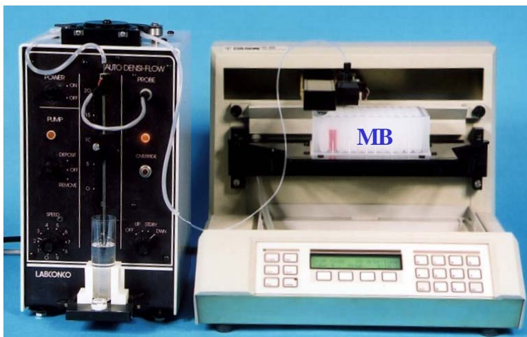
Figure 8: Integrated automatic gradient harvesting and fractionation. The gradient is shown being collected from the meniscus using a Labconco Auto Densi-flow, fractionated in a Gilson FC205 fraction collector into a 96-well Greiner Bio-One MasterBlock multiwell plate.
